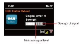
The indicator on the signal bar shows the minimum acceptable signal level.
